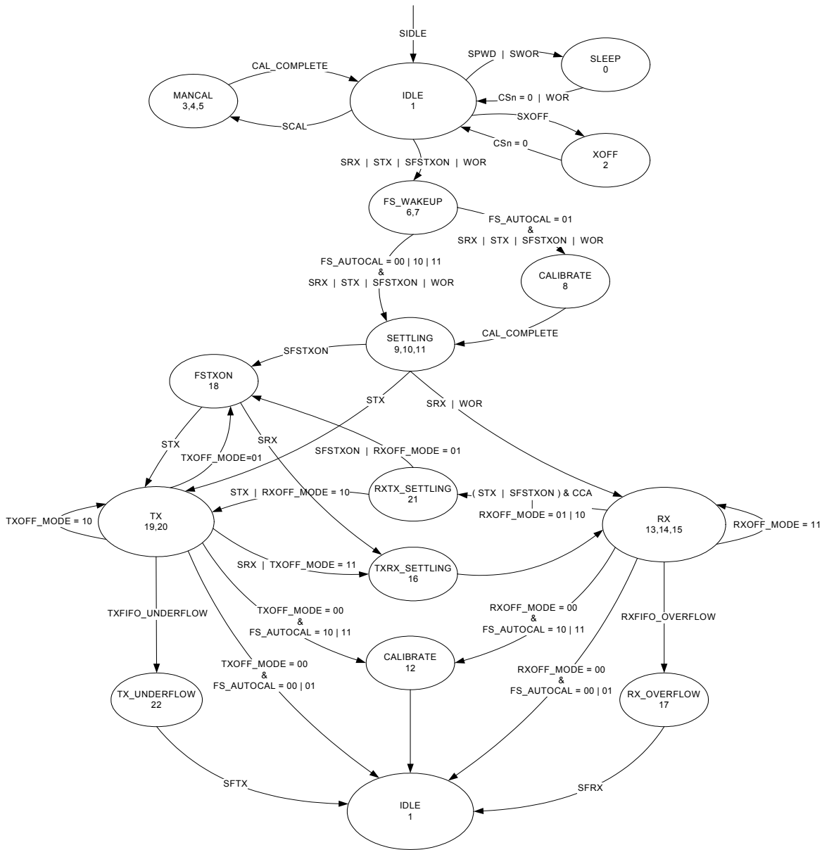
Figure 16: Complete Radio Control State Diagram
